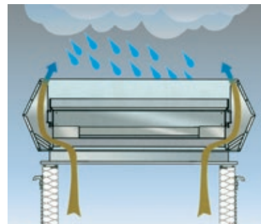
functions SMOKEJET® R/SMOKEJET® RD: fair weather, rain-proof ventilation and SHEV systems illustration of ventilation in case of rain
